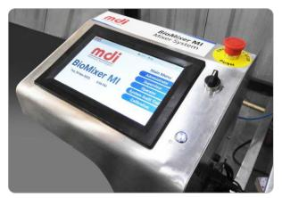
Control panel with capacitive touch screen display
